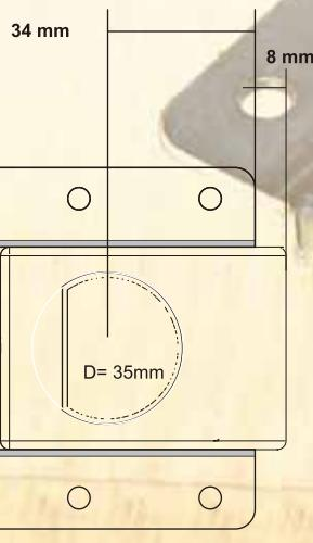
This versatile sliding latch can be used in a variety of functions such as service hatches, doors, lids, etc. Special care has been taken in the development of this product to keep it flat, thereby taking up as little space inside as possible.
